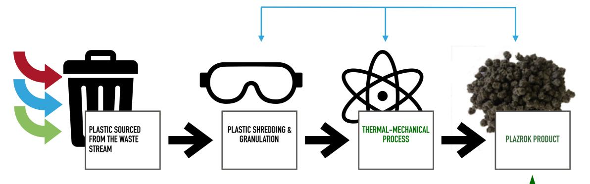
PLAZROK IS MANUFACTURED USING A COMPLETE CO-MINGLED MIX OF WASTE PLASTIC THAT WOULD OTHERWISE END UP IN LANDFILL
